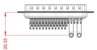
40A (CURRENT) POWER/CO-AX CONTACT RATING: (IF PRESENT) SIGNAL CONTACT CURRENT RATING: 5A PER CONTACT SIGNAL CONTACT RESISTANCE:  $10m\Omega$  MAX. **INSULATOR RESISTANCE:** 5000MΩ min. DIELECTRIC
