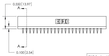
0.420 [10.67] Card Slot 0.34 [8.53] 0.31 7.77 Point of Contact 0.550 13.97 0.300 [7.62] SECTION A-A
