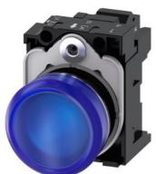
Indicator light, 22 mm, round, metal, shiny, blue, lens, smooth, with holder, LED module with integrated LED 110 V AC, spring-type terminal, with laser labeling, upper case and lower case, always upper case at beginning of line
