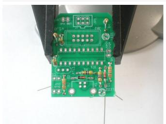
Next are the zener diodes. Diodes are directional so make sure to put them in as shown. There's a white stripe on the PCB drawing that matches the black stipe on the glass diode.
