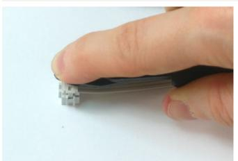
Do not use needlenose pliers to try to press the pieces together. You have to have very flat pressure from both sides
