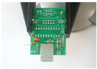
The next parts are the USB connector (big silver part), the 12.00MHz ceramic oscillator (the three pin part) and the ceramic capacitor (the small yellow part).
