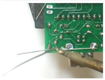
Solder and clip the two LEDs.
