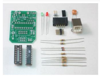
Check the kit to verify you have all the parts necessary (the 0.1uF capacitor is missing, oops!).
