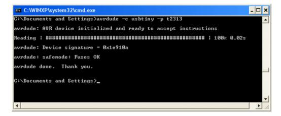
Using it is simple, just indicate usbtiny as the programmer type. The port option is ignored as it always uses USB.
