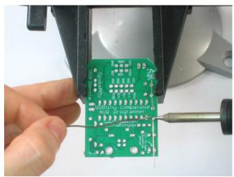
Solder the legs. Hold the tip of iron against the wire leg and the metal ring at the same time, after 2 counts, poke the solder in till it creates a nice pool. Then remove the solder, wait a half count, then remove the iron. Do this for both legs.
