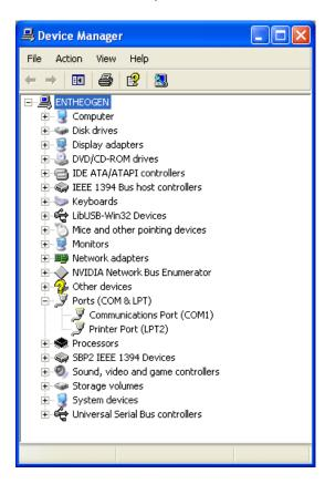
Under ports you'll see a list of COM ports. Both of the virtual ports we're making have to be between COM1 and COM9. Looks like only COM1 is being used.
