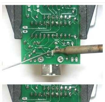
Solder in the three-pins of the oscillator and all 6 pins of the USB connector. Make sure to not bridge any of the square-pins and put plenty of solder on the mechanical tabs. These provide the resistance when you plug in a cable so it's important that they are soldered well, as shown here.
