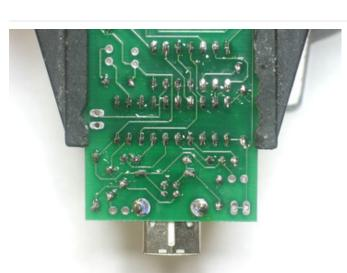
Although they are short, you should clip the pins to the oscillator if possible, to make sure they dont bend over and touch another component.
