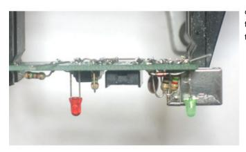
The LEDs are also supposed to be very close to the top of the enclosure, so that you can see the light through the drilled holes, when you bend the leads, make sure the LEDs stick out about 1/2" above the PCB.
