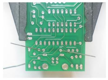
Bend the wire legs so that when the board is flipped over, it won't fall out.
