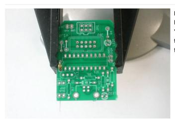
Place the first component: the 10K resistor as shown. Resistors are non-directional, so you can put them in 'either' way and they'll work fine. When you put the legs through the PCB, bend them out so when the PCB is flipped it wont fall out.
