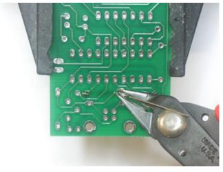
Next, clip the excess leads using the diagonal cutters. Clip right above the top of the solder joint.
