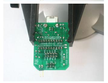
The 10-pin box header has a notch which should match the notch in the PCB graphic. (here it's closest to the microcontroller socket).
