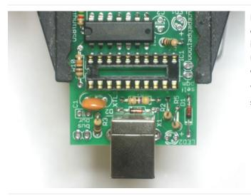
Next is the USB connector and the 12.00MHz ceramic oscillator. The USB connector is what we use to plug into the computer, the oscillator makes sure the USBtiny microcontroller runs at the precise rate necessary to communicate at the very picky USB protocol rates.
