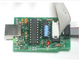
Plug in the two cables as shown, the red stripes on top and so that the cables don't bend over the plug (the case wont fit).
