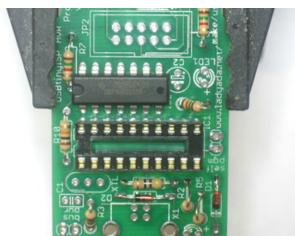
Next to be placed is the 74AHC125 buffer. This chip does a level-shifting conversion on signals from the USBtiny microcontroller to the device being programmed. This way you can safely program chips that vary from 1.8V to 5.5V voltage.
