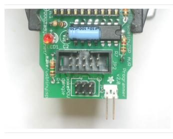
Almost done! The last set of parts are the headers for the cables, and the jumper header. The 10-pin box header has a notch in it, make sure it matches up with the silkscreen, as shown.
