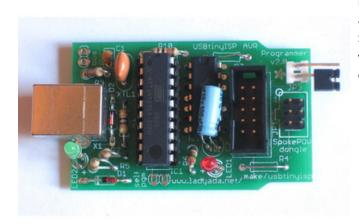
If you're not using the USBtiny to talk to a SpokePOV kit, and if you are using a target that has some load on the SCK and MOSI pins, you may need to replace R4 and R7 with jumpers as the 1.5K resistors will have trouble driving the load!
