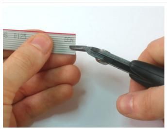
It's hard to find 6-conductor ribbon cable so you may end up with 10-conductor wire. (The kit ships with 6conductor) If so, just use your diagonal cutters (or a knife) to cut a notch so that the red stipe is on the 6conductor side.
