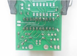
Tack two opposite corners of the socket, to keep it in place, and then solder all the pins.
