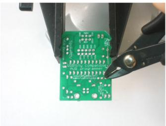
Use the diagonal cutters to clip the legs off just above the solder joint.
