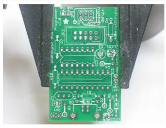
Next, get ready by placing the PCB in a vise so that you can easily place and solder the parts in!
