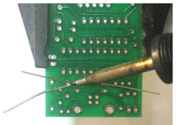
Next, with your soldering iron, solder each of the resistor legs. Place the tip of the iron against both the pad (ring) and lead (leg) and after a few counts, touch the solder in, to make a nice joint.
