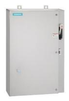
Non-reversing motor starter Size 1 Three phase full voltage Solid-state overload relay OLRelay amp range 0.75-3.4A Combination type 30Amp non-fusible disconnect Encl NEMA type 4X 316 S-steel Water/dust tight non-corrosive Extra-wide enclosure
