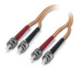
Assembled FO cable, zip cord cable, multi-mode fiberglass 50/125  $\mu$ m, OM2, plug: B-FOC (ST)/B-FOC (ST), degree of protection: IP20, for installation in cable ducts or control cabinets, length: 1 m
