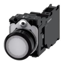
Illuminated pushbutton, 22 mm, round, plastic, white, pushbutton, flat, momentary contact type, with holder, 1 NO+1 NC, LED module with integrated LED 24 V AC/DC, spring-type terminal, with laser labeling, upper case and lower case, Always upper case at the beginning of the word
