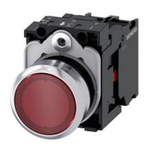
Illuminated pushbutton, 22 mm, round, metal, shiny, red, pushbutton, flat, momentary contact type, with holder, 1NC, LED module with integrated LED 110 V AC, screw terminal, with laser labeling, upper case and lower case, Always upper case at the beginning of the word
