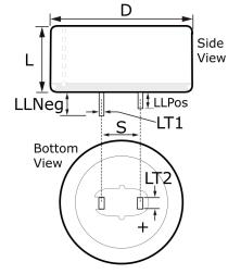
General InformationSeriesFSDescriptionRadial Cylindrical Double Layer CapacitorRoHSYesAEC-Q200NoComponent Weight2.6 gMiscellaneousDischargeValue = 0.072 F.
