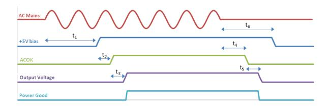
Typical timing values:  $t_1 \phi$  300 ms,  $t_2 \phi$  50 ms,  $t_3 \phi$  25 ms,  $t_4 \phi$  15 ms,  $t_5 = 5$  ms (minimum),  $t_6 \phi$  100 ms
