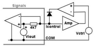
It is <u>not</u> recommended to use remote voltage/current programming in normal parallel mode.
