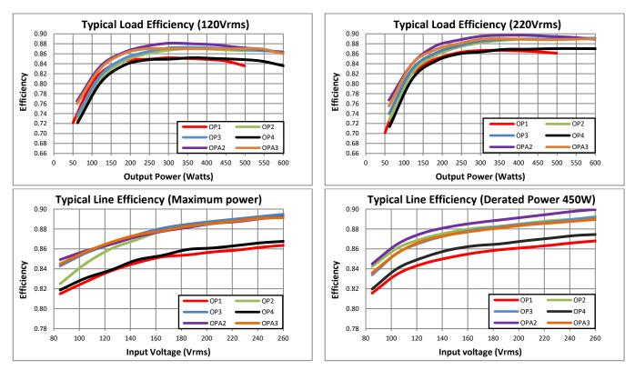
An estimate of the efficiency for any particular system may be obtained from these graphs using the procedure outlined in the example below.
