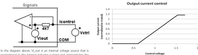
In the diagram above, VI\_out is an internal voltage source that is proportional to the internal inductor current and <u>approximates</u> the equation,
