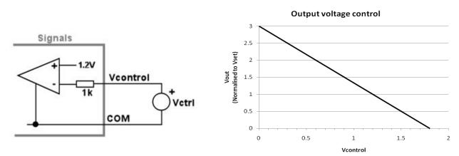
The output voltage can be controlled from 0% to 300% of the preset voltage using this control method. However, care must be taken to ensure the output voltage does not exceeed the OVP level, as this is considered a safety hazzard and will latch the entire unit off. To determine the level of control voltage that will trigger OVP, insert Vovp into the equation above.
