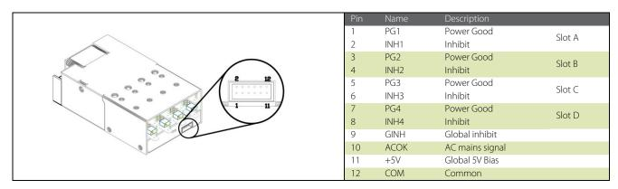
Note that for modules requiring more than 1 slot, the INHx and PGx use the highest number available for x. The other controls will have no function. E.g. For an OPA2 fitted in slots AB, INH1 & PG1 have no function while INH2 and PG2 provide the usual functions for the module.
