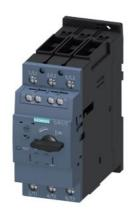
Special type Circuit breaker size S2 for motor protection, CLASS 10 A-release 35...45 A N-release 650 A screw terminal Standard switching capacity with transverse auxiliary switches 1 NO+1 NC Ambient temperature -50 °C 250 switching cycles
