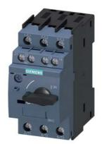
Circuit breaker size S00 for transformer protection A-release 0.7...1 A N-release 21 A screw terminal Standard switching capacity with transverse auxiliary switches 1 NO+1 NC  $\,$
