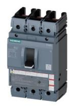
circuit breaker 3VA5 UL frame 250 breaking capacity class C 100kA @ 480V 3-pole, line protection TM210, FTFM, In=110A overload protection Ir=110A fixed short-circuit protection Ii=10 x In UL 489 SB (naval), 50° C without connection
