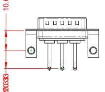
10A (CURRENT) POWER/CO-AX CONTACT RATING: (IF PRESENT) SIGNAL CONTACT CURRENT RATING: 5A PER CONTACT SIGNAL CONTACT RESISTANCE:  $10m\Omega$  MAX. **INSULATOR RESISTANCE:**
