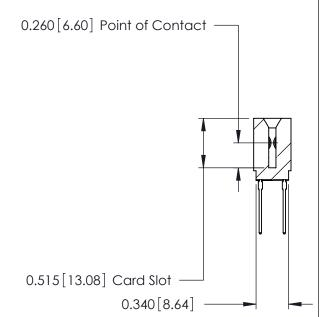
ACAD REFERENCE NO. 746-ENG MASTER 746 Series Ultra-Mate Card Edge Connector - Press Fit DRAWN: J.LEE DATE: AUG 20/09 Part Number: 746-032-540-201 CHECKED: DATE: **EDAC INC** SCALE: SHEET 1 OF 1 THESE DRAWINGS AND SPECIFICATIONS ARE THE PROPERTY OF EDAC INC.,AND TORONTO, ONTARIO SHALL NOT BE REPRODUCED, OR COPIED DRAWING NUMBER **ISSUE** CANADA OR USED AS THE BASIS FOR THE 746-ENG MASTER MANUFACTURE OR SALE OF APPARATUS YOUR CONNECTION TO QUALITY & SERVICE WITHOUT WRITTEN PERMISSION.
