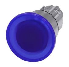
Illuminated mushroom pushbutton, 22 mm, round, metal, shiny, blue, 40 mm, latching, pull-to-unlatch mechanism, Z=50-unit packaging
