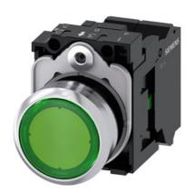
Illuminated pushbutton, 22 mm, round, metal, shiny, green, pushbutton, flat, momentary contact type, with holder, 1NO, LED module with integrated LED 110 V AC, spring-type terminal, with laser labeling, inscription or symbol Customer-specific selection with SIRIUS ACT configurator (CIN)
