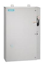
Non-reversing motor starter Size 0 Three phase full voltage Solid-state overload relay OLRelay amp range 0.75-3.4A 208VAC 60HZ coil Combination type 30Amp non-fusible disconnect Encl NEMA type 4X 316 S-steel Water/dust tight non-corrosive Extra-wide enclosure
