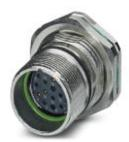
Device connector for rear wall, straight, shielded: yes, for standard and SPEEDCON interlock, M23, No. of pos.: 16+2+PE, type of contact: Socket, Crimp connection, Axial seal, Central fixing
