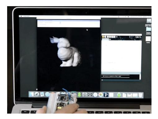
Also notice in the upper right corner of the dialog box at the top that the calibration of each sensor is displayed. It's important to calibrate the BNO055 sensor so that the most accurate readings are retrieved. Each sensor on the board has a separate calibration status from 0 (uncalibrated) up to 3 (fully calibrated). Check out the video and information from this guide for how to best calibrate the BNO055 sensor (https://adafru.it/kA1).
