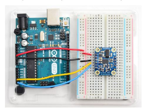
If you're using a Genuino Zero or Arduino Zero with the built in EDBG interface you may need to use I2C address 0x29 since 0x28 is 'taken' by the DBG chip
