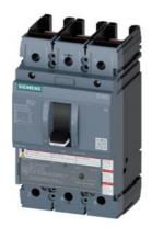
circuit breaker 3VA5 UL frame 250 breaking capacity class C 100kA @ 480V 3-pole, line protection TM210, FTFM, In=100A overload protection Ir=100A fixed short-circuit protection Ii=10 x In UL 489 SB (naval), 50° C without connection
