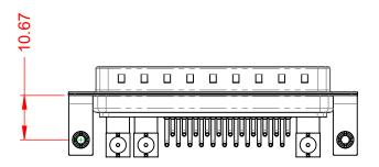
POWER/CO-AX CONTACT RATING: (IF PRESENT) SIGNAL CONTACT CURRENT RATING: 5A PER CONTACT SIGNAL CONTACT RESISTANCE:  $10m\Omega$  MAX. **INSULATOR RESISTANCE:** 5000MΩ min.
