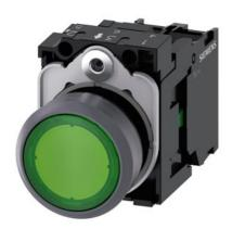
Illuminated pushbutton, 22 mm, round, plastic with metal front ring, green, pushbutton, flat, momentary contact type, with holder, 1NO, LED module with integrated LED 110 V AC, screw terminal, with laser labeling, upper case and lower case, always upper case at beginning of line
