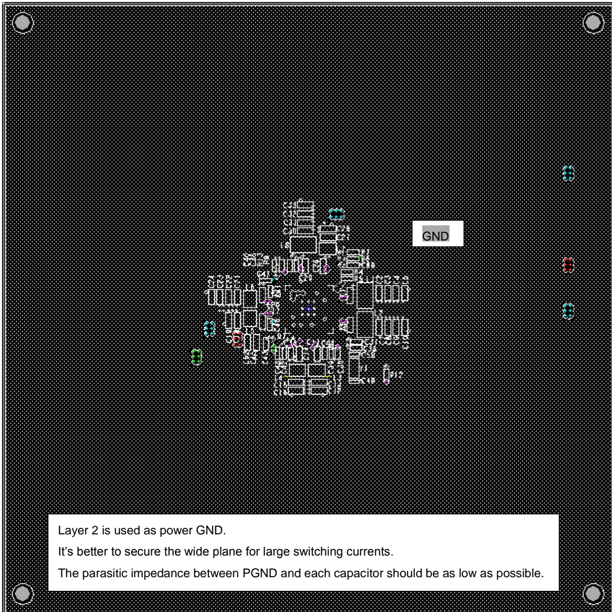
Figure 4.7 BD71837MWV Reference Board Outline (Layer 2)
