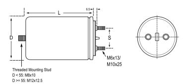
General Information Series C44A Dielectric Metallized Polypropylene Style RoHS With Exemptions **REACH** SVHC (Pb - CAS 7439-92-1) cc1c1ec4-db9e-4815-b26b-e8a34ddfb776 SCIP Number Lead Threaded Studs M6 AEC-Q200 No Component Weight 256 g Thermal Resistance = 2.7 C/W. Miscellaneous
