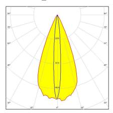
Dimensions: 32.0 mm x 32.0 mm Height: 19.05 mm ~20° + 40° oval beam. Assembly
