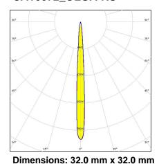
**Height: 19.05 mm**~9° spot beam beam. Optimized for high-power 3535 size LED packages. Assembly with holder and installation tape.
