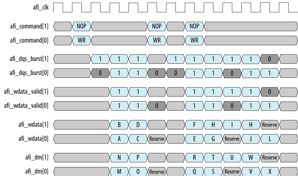
Figure 36. AFI Write Data with CRC Half-Rate, wlat=2
