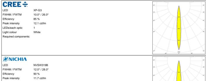
LEDs/each optic 1 Light colour White Required components:
