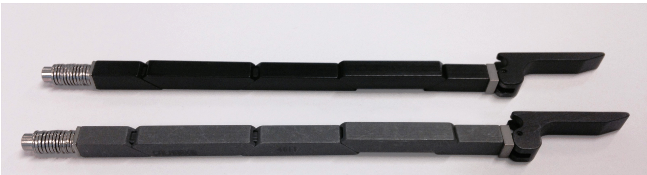
Top: Sample with black anodize finish only, no dry film lube (future) Bottom: Sample with black anodize and dry film lube finish (current)
