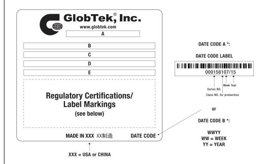
A=Medical/ITE/Household use Power Supply B=P/N: (料号) TR9KB3865T00NAIMR6B C=Model (型号) GTM96300-2307.5-1.55-T2 D=Input (输入) 100-240V~, 50-60 Hz, 1A E=Output (输出)5.95 V == 3.86 A, 23.0W
