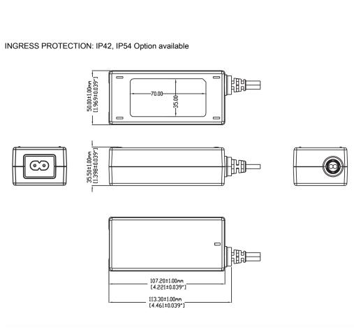
Alternative housing with waterproof barrier. Product PN# ends with suffix "RG"
