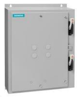
Duplex starter w/o alternator Size 1.75 Three phase full voltage Solid-state overload relay OLR amp range 10-40A Combination type Two 60A disconnect switches Enclosure NEMA type 1 Indoor general purpose use
