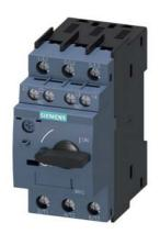
Circuit breaker size S00 for transformer protection A-release 2.8...4 A N-release 82 A screw terminal Standard switching capacity with transverse auxiliary switches 1 NO+1 NC
