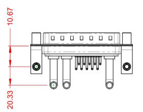
40A (CURRENT) POWER/CO-AX CONTACT RATING: (IF PRESENT) SIGNAL CONTACT CURRENT RATING: 5A PER CONTACT SIGNAL CONTACT RESISTANCE:  $10m\Omega$  MAX. **INSULATOR RESISTANCE:**
