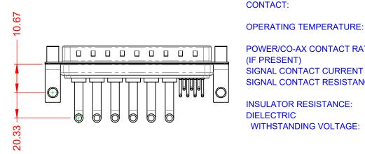
30A (CURRENT) POWER/CO-AX CONTACT RATING: (IF PRESENT) SIGNAL CONTACT CURRENT RATING: 5A PER CONTACT SIGNAL CONTACT RESISTANCE:  $10m\Omega$  MAX. **INSULATOR RESISTANCE:** 5000MΩ min.
