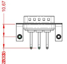
10A (CURRENT) POWER/CO-AX CONTACT RATING: (IF PRESENT) SIGNAL CONTACT CURRENT RATING: 5A PER CONTACT SIGNAL CONTACT RESISTANCE:  $10m\Omega$  MAX. **INSULATOR RESISTANCE:**
