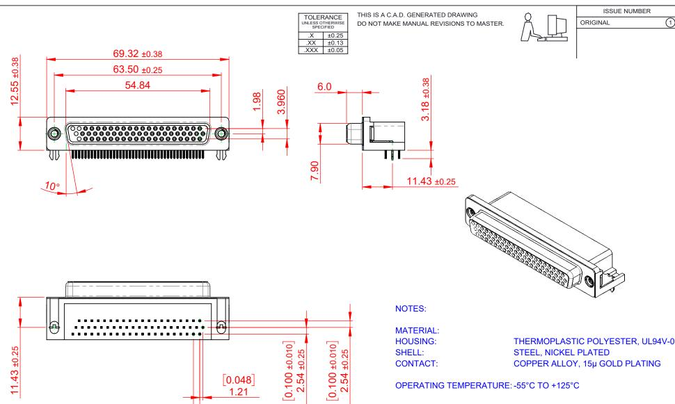
**CURRENT RATING:** 3A PER CONTACT  $25m\Omega$  MAX. **CONTACT RESISTANCE: INSULATOR RESISTANCE:** 5000MΩ min.
