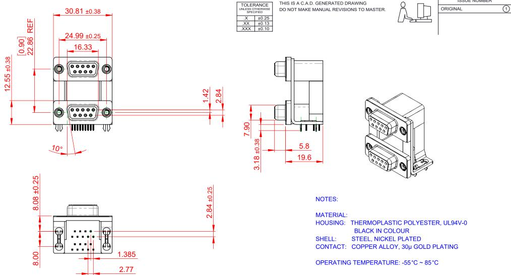
CURRENT RATING:3A PER CONTACTCONTACT RESISTANCE: $25m\Omega$  MAX.INSULATOR RESISTANCE: $5000M\Omega$  min.DIELECTRICWITHSTANDING VOLTAGE:100V AC rms
