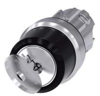
RONIS key-operated switch, 22 mm, round, metal, shiny, lock number 455, with 2 keys, 2 switch positions O-I, latching, actuating angle 90°, 10:30h/13:30h, key removal I, with laser labeling, upper case and lower case, always upper case at the beginning of the word
