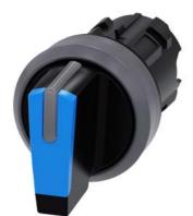
Selector switch, illuminable, 22 mm, round, plastic with metal front ring, blue, selector switch, short, 3 switch positions I>O<II, momentary contact on the left, latching on the right, actuating angle 2x45°, 10:30h/12h/13:30h, with laser labeling, upper case and lower case, always upper case at beginning of line
