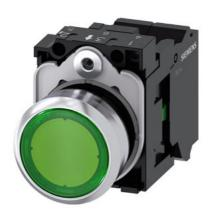
Illuminated pushbutton, 22 mm, round, Metal, shiny, green, pushbutton, flat, momentary contact type, with holder, 1NO, LED module with integrated LED 230 V AC, spring-type terminal, with laser labeling, symbol number according to, ISO 7000 or IEC 60417
