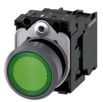
Illuminated pushbutton, 22 mm, round, plastic with metal front ring, green, pushbutton, flat, momentary contact type, with holder, 1NO, LED module with integrated LED 110 V AC, screw terminal, with laser labeling, inscription or symbol Customer-specific selection with SIRIUS ACT configurator (CIN)
