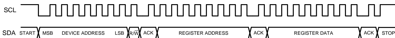
Figure 26. Example I 2 C Write Cycle
