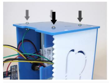
Tighten all four screws using a screwdriver (finger-tight).
