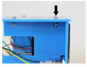
Lower the side piece into place...slots should fit into corresponding tabs.
