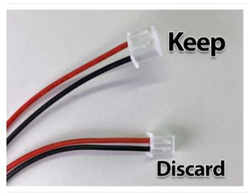
**Cut** the **red/black power cable** in **half**. This cable has a different plug at each end. We want to **keep the wider of the two plugs** for the printer; the other can be discarded or tossed in your spare bits drawer.
