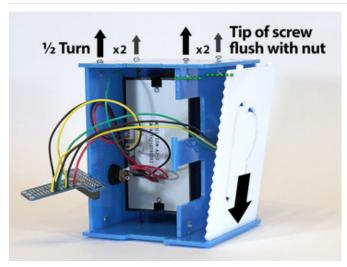
Slot one end of the front piece into the side of the case. The "torn receipt" effect should be at the bottom.
