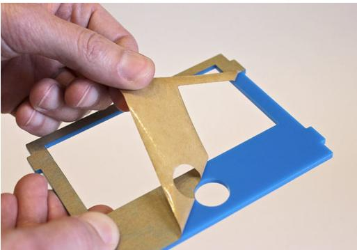
After peeling, the parts may have a little bit of paper soot on them from laser cutting. Wiping off may suffice, or they can be **washed** with soap and water...but be absolutely certain that everything is **completely dry** before assembling components in the case!
