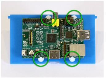
If you have an early "rev1" Raspberry Pi board without mounting holes, this can be installed using a set of four board edge mounts (http://adafru.it/1116) (sold separately, not included in kit).
