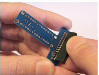
Normally the Cobbler would have a header soldered to the top, but we're doing something different with this kit: the socket sits on the *underside* of the board.
