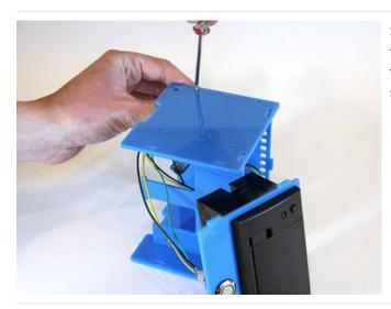
Scoot the printer out a bit so you can reach theremaining t-slots. Insert a nut into one of the slots, set the second side of the case into position and install a screw.
