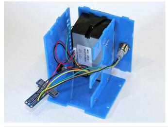
Stand the partial case up on its side and move the top piece (with button and thermal printer attached) roughly into position. Don't fit this into the slots yet, just an approximate position.
