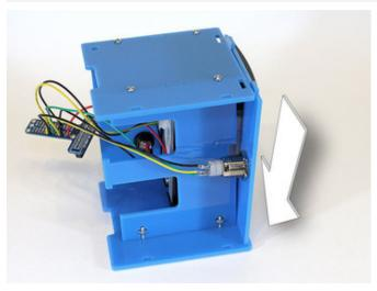
Slot one end of the top/printer piece into position. But with both sides in place, the slots at the other end are now blocked. The next few steps take care of all this...
