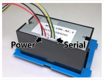
Connect the serial cable and power from the DC jack, noting the labels on the bottom of the printer. The connectors are identical and it's easy to get these switched around.
