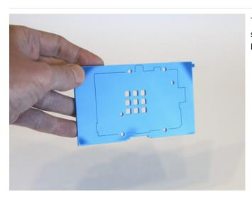
The bottom piece is scored on one side, with an outline showing the placement and orientation of the Raspberry Pi board.
