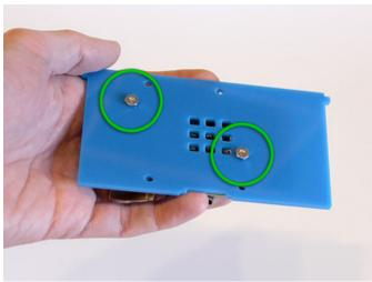
Position the bottom plate over the Raspberry Pi (remember, the scored side should face the board) and secure in place with two #4-40 nuts. Tighten the screws from the other side using a small screwdriver and gentle pressure — don't crank the screws down hard or you'll crack the case!
