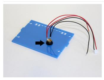
Secure the DC jack from the other side with the included nut. You'll need to fish the wires through this to get it into place.
