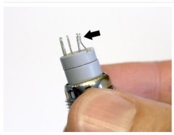
Using finger pressure or small pliers (gently!), smoosh the last two pins (COMMON and LED –) close together. We need to loop a single wire through both of them...
