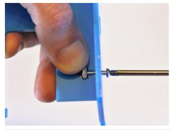
Use a screwdriver to turn the nut into place. Just "finger tight" is good for now...in subsequent steps we'll be loosening certain screws anyway.
