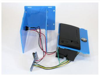
You should now have four nuts and screws installed in one side piece, holding the back and center support.
