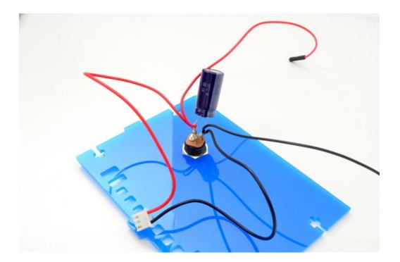
MAKE SURE THE NEGATIVE (shorter) LEG OF THE CAPACITOR IS CONNECTED TO BLACK/GND AND THE POSITIVE LED IS CONNECTED TO RED/5VDC.
