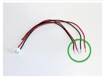
Strip about 1/4" insulation from the red and black wires on the power cable <u>and</u> the spare wires.
