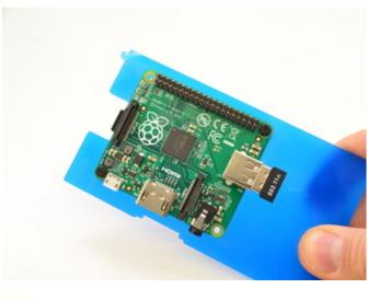
Push out the laser cut holes and mount the Raspberry Pi Board to the bottom plate using the included plastic #4-40 screws
