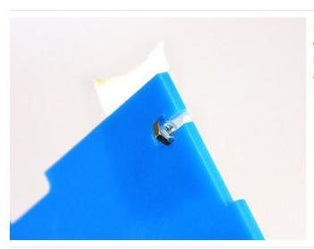
If holding the part and the nut simultaneously is a dexterity challenge, you can instead use a bit of tape to provide a temporary hold for the nut. This can be peeled away once the corresponding screw is in place.
