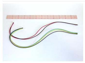
In the plastic baggie accompanying the thermal printer should be two cables. The power cable has two conductors: red and black. The data cable has three conductors: green, yellow and black.
