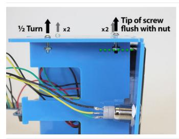
Loosen two of the lower screws about 1/2 turn.
