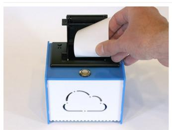
Pull up the top lever to access the paper compartment. Insert a roll of thermal receipt paper and push the lid closed while feeding the end of the paper through the slot.
