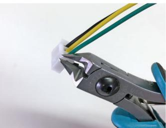
Use wire cutters to clip the side "wings" off the plug at one end of the data cable.
