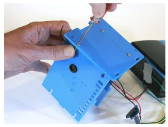
Connect the same side piece to the case back, using two nuts and screws as before.
