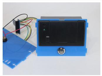
Being mindful of the wires and other attached components, slide the thermal printer through the large slot on the top case piece, with the feed button toward the BACK (the silver button is toward the front).
