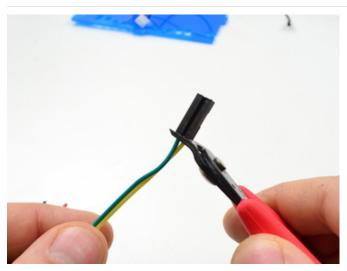
Next, grab the female/female jumper wires and cut off the connector at **one end** of each of the following colors:
