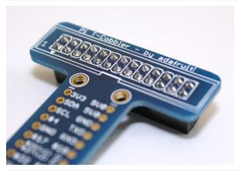
Once the header is straight, the rest of the pins can be soldered.
