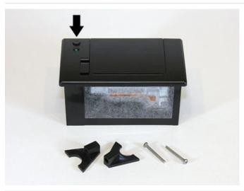
The parts baggie included with the thermal printer contains two triangle-shaped brackets and two long screws. These will hold the printer inside the case.
