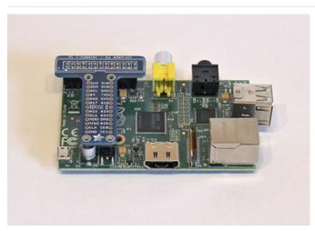
After soldering (and allowing some time to cool), you can test fit the Cobbler on the Raspberry Pi. Gently pry it off with your fingers afterward...more soldering lies
