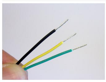
Strip about 3/8" of insulation from the end of three of the spare wires: **BLACK**, **YELLOW** and **GREEN**. Twist the ends a bit to keep the strands from fraying.
