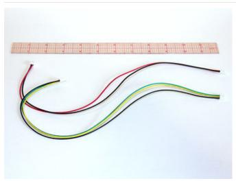
In the plastic baggie accompanying the thermal printer should be two cables, a bit over a foot long. The **power cable** has **two** conductors: red and black. The **data cable** has **three** conductors: green, yellow and black.
