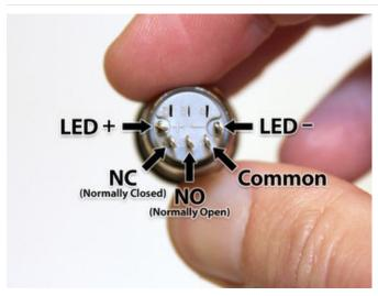
Looking at the back of the button, with the pins arranged in a "smile," the functions from left to right are:
