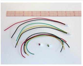
After cutting, you should have two cables, each about 7 inches long, both with a "wide" connector: one for power (red and black) and one for data (green, yellow and black).
