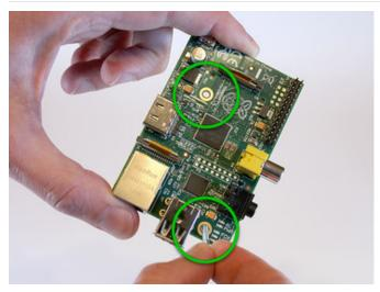
All but the earliest Raspberry Pi boards have two mounting holes. Insert a 1/2" #4-40 screw into each of these holes from the top of the board.
