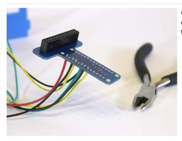
Once all the wires have been soldered, you can trim any excess on the underside so that nothing accidentally touches the Pi board.
