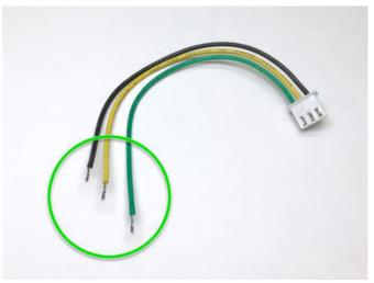
Strip about 1/4" insulation from the three wires of the serial data cable.
