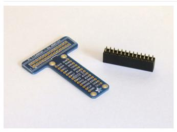
First we'll be joining the T-Cobbler board and 26-pin socket.
