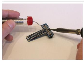
Tack the header in place by soldering just one pin (any will do) on the top side of the board. Notice we're soldering on the <u>label</u> side for this step.
