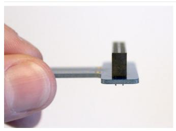
Check that the header is straight and square. If not, heat the one soldered pin and realign the header.
