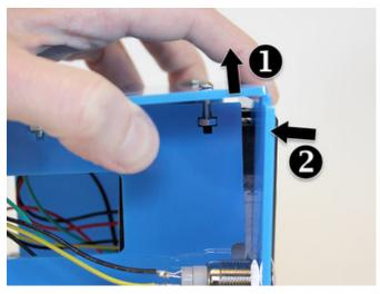
Lift the side of the edge piece. There should be just enough "play" for the tabs from the top piece to fit underneath. Press the printer piece into position.
