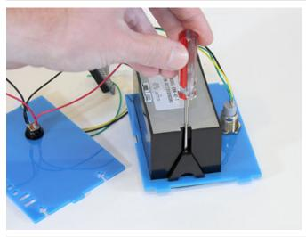
Set the printer and top piece face-down and insert the two brackets and screws. Use a small screwdriver to secure these in place. Use gentle pressure! Cranking these down tightly can crack the case.
