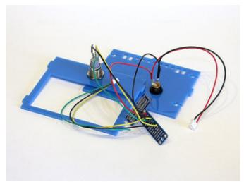
The button and power wires are now soldered to the Cobbler using the wiring diagram.
