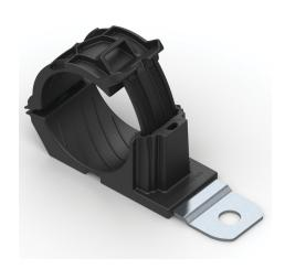
Ratchet P-Clamp, 1.42 - 2.0" Bundle Dia, 180° Short, 0.26" Hole Dia, PA66HIRHSUV/ST/ZN, Black, 20/bag
