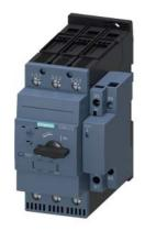
Circuit breaker size S2 for motor protection, CLASS 10 with overload relay function A-release 54...65 A N-release 845 A screw terminal Standard switching capacity
