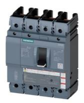
circuit breaker 3VA5 UL frame 250 breaking capacity class M 35kA @ 480 V 4-pole, line protection TM240, ATAM, In=200A overload protection Ir=160A...200A short-circuit protection Ii=5...10 x In N conductor protection 100% without connection
