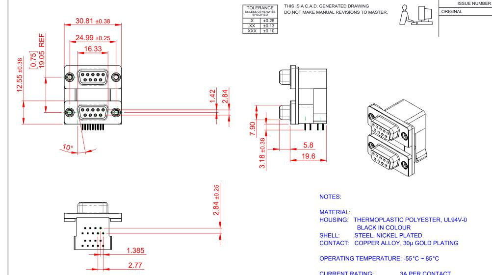
**CURRENT RATING: 3A PER CONTACT** 25mΩ MAX. CONTACT RESISTANCE: INSULATOR RESISTANCE: 5000MΩ min. DIELECTRIC WITHSTANDING VOLTAGE: 1000V AC rms
