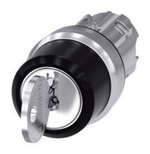
RONIS key-operated switch, 22 mm, round, metal, shiny, lock number 455, with 2 keys, 3 switch positions I>O<II, momentary contact type, actuating angle  $2x45^{\circ}$ , 10:30h/12h/13:30h, key removal O, with laser labeling, upper case and lower case, always upper case at beginning of line
