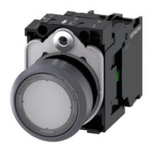
Illuminated pushbutton, 22 mm, round, plastic with metal front ring, clear, pushbutton, flat, momentary contact type, with holder, 1NO, LED module with integrated LED 110 V AC, screw terminal, Z=20-unit packaging
