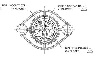
REDUCED DIA. WIRE SEAL SEALED PANEL MOUNT
